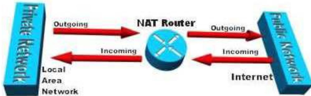
The operation of NAT Router(NAT box) is as shown above. Assume that within the company premises every machine has a unique address of the form 10.x.y.z. However, when a packet leaves the company premises, it passes through a NAT box that converts the internal IP source address, to the company's true IP address and sends it to the destination.
