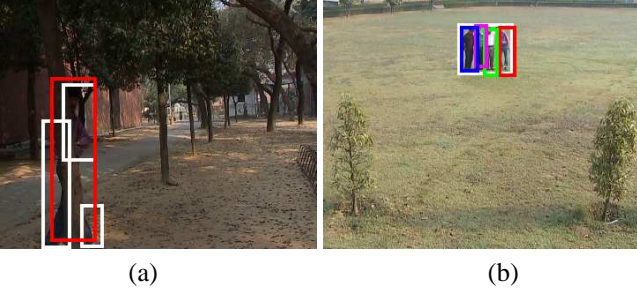
Figure 2. Cases of occlusions. (a) Partial occlusion: agent occluded by tree is visible as three fragmented blobs; in this state, the agent is recognized, but its visual characteristics are not updated. (b) Crowding: multiple agents merge to form a single blob. Each agent in the blob must be partially visible (otherwise it is flagged as disappear ).
